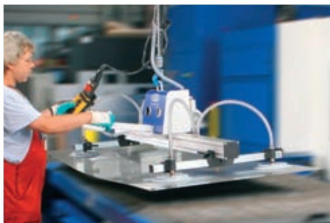
VacuMaster Basic, charge 250 kg, manipulation horizontale
