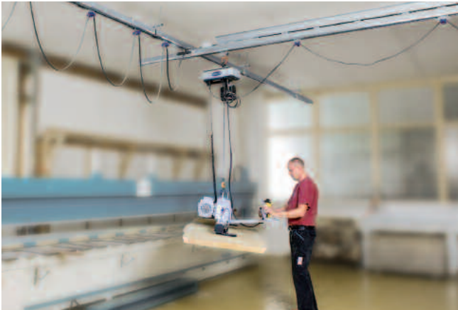
Steel crane system with one beam, 250 kg, 6x12 m
