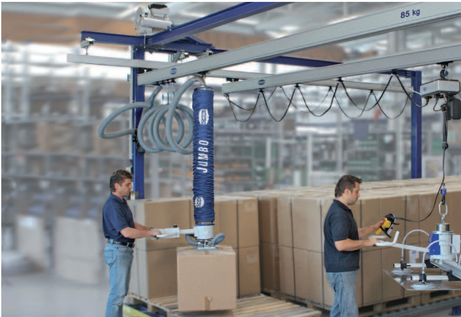
Aluminium crane system with one beam, 85 kg or 150 kg load, 2x6 m or 4x6 m
