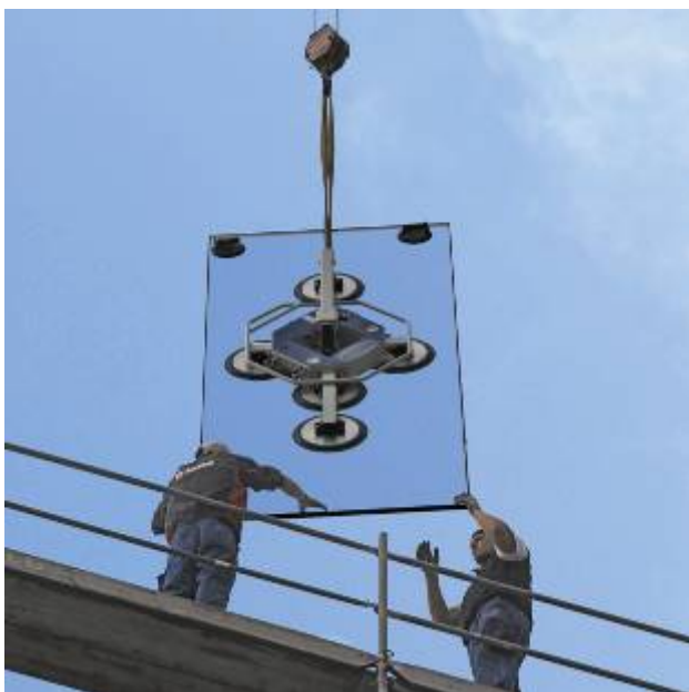
VacuMaster Glass, maximum load 450 kg, handling glass sheets
