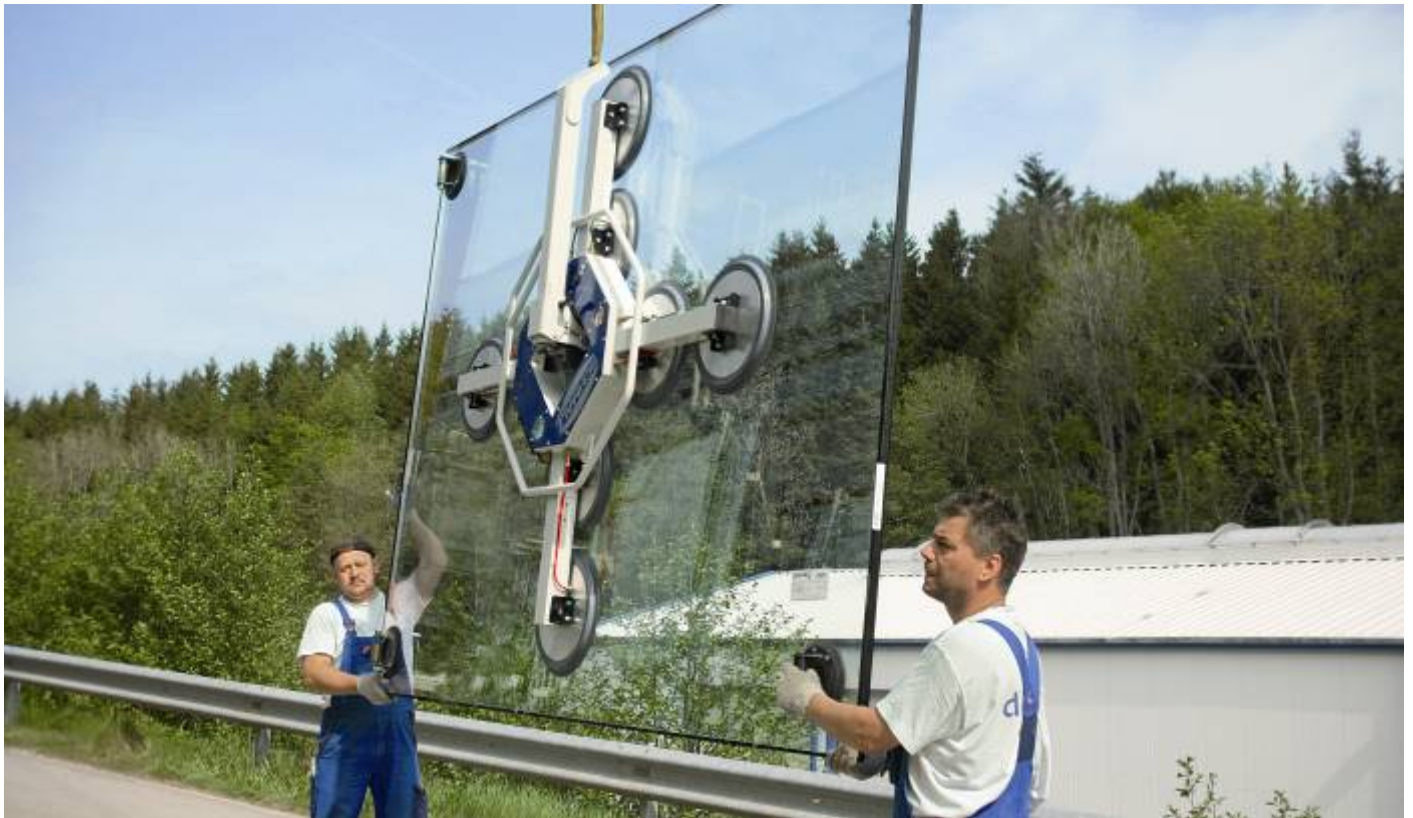
VacuMaster Glass, maximum load 600 kg, for handling of glass sheets
