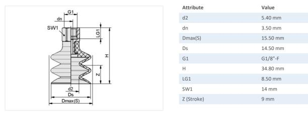
Note: Acceptable dimensional tolerances for elastomer parts concerning to DIN ISO 3302-1 M3
