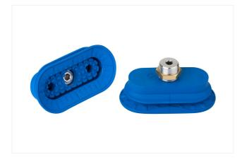
Dimensions (LxB): 80 x 40 Suction cup material: High temperature material HT1 Material hardness [Shore A]: 60 Shore A Nipple material: Aluminum Connection: G3/8-AG
