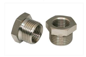
Thread G1: G3/8"-M Thread G2: G1/4"-F Material: Brass Surface: nickel plated Length L: 5 mm
