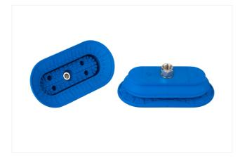
Dimensions (LxB): 140 x 70 Suction cup material: High temperature material HT1 Material hardness [Shore A]: 60 Shore A Nipple material: Nickel plated Connection: G1/4-IG Number of folds: 1.5
