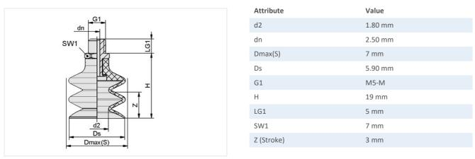
Note: Acceptable dimensional tolerances for elastomer parts concerning to DIN ISO 3302-1 M3
