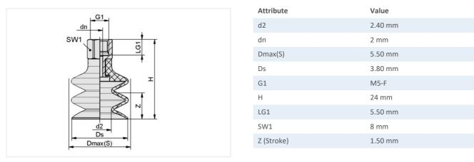
Note: Acceptable dimensional tolerances for elastomer parts concerning to DIN ISO 3302-1 M3
