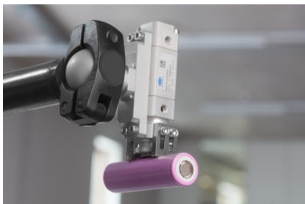
Magnetic gripper for handling hard case steel cells
