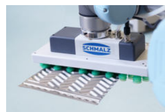
Handling of battery modules in the pack assembly
