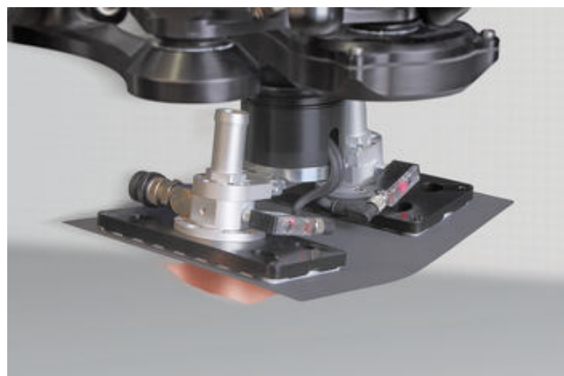
Special gripper STGG for handling anodes
