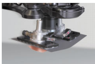
Handling of electrodes and separators in cell production
