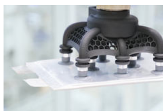
Handling of pouch cells in module assembly
