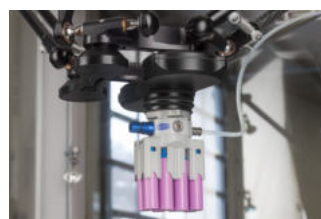
Handling of round cells in module assembly
