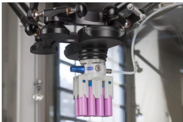
Customer-specific grippers, adapted to the size and quantity of the round cells
