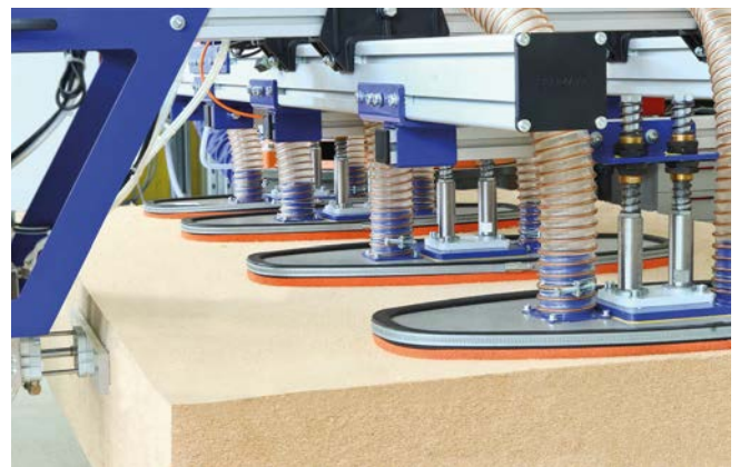
Construction materials | Vacuum suction spider SSP being used to handle and separate porous sheets of insulation
