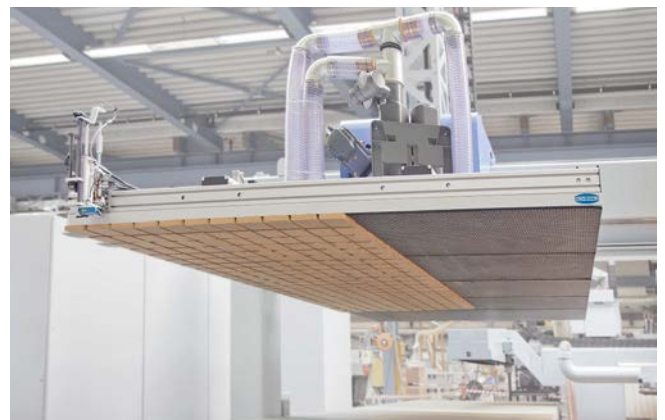
Schmalz Nesting Gripper SPZ-NG for destacking complete layers of workpieces during nested manufacturing
