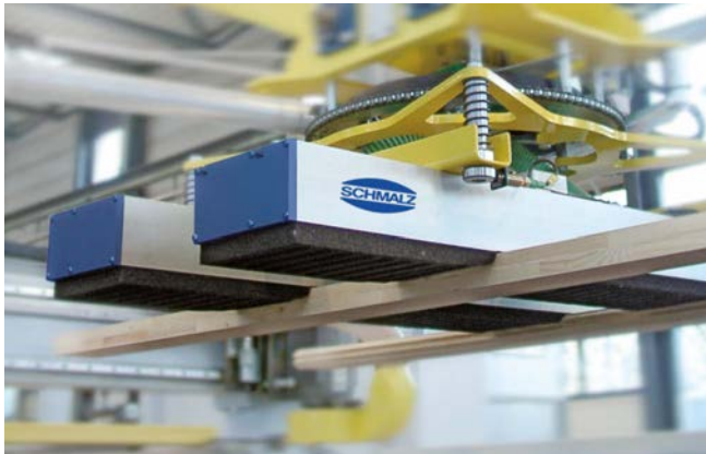
Vacuum area gripping system SBX
