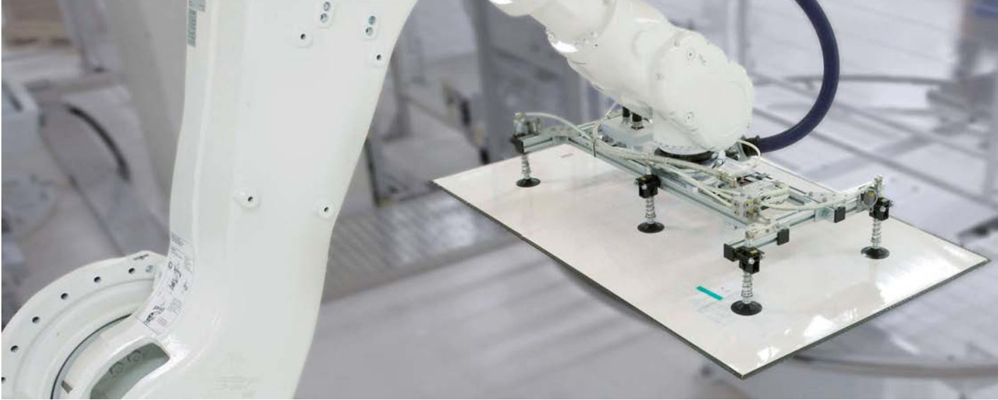
Solar | Vacuum suction spider SSP being used to handle module glass
